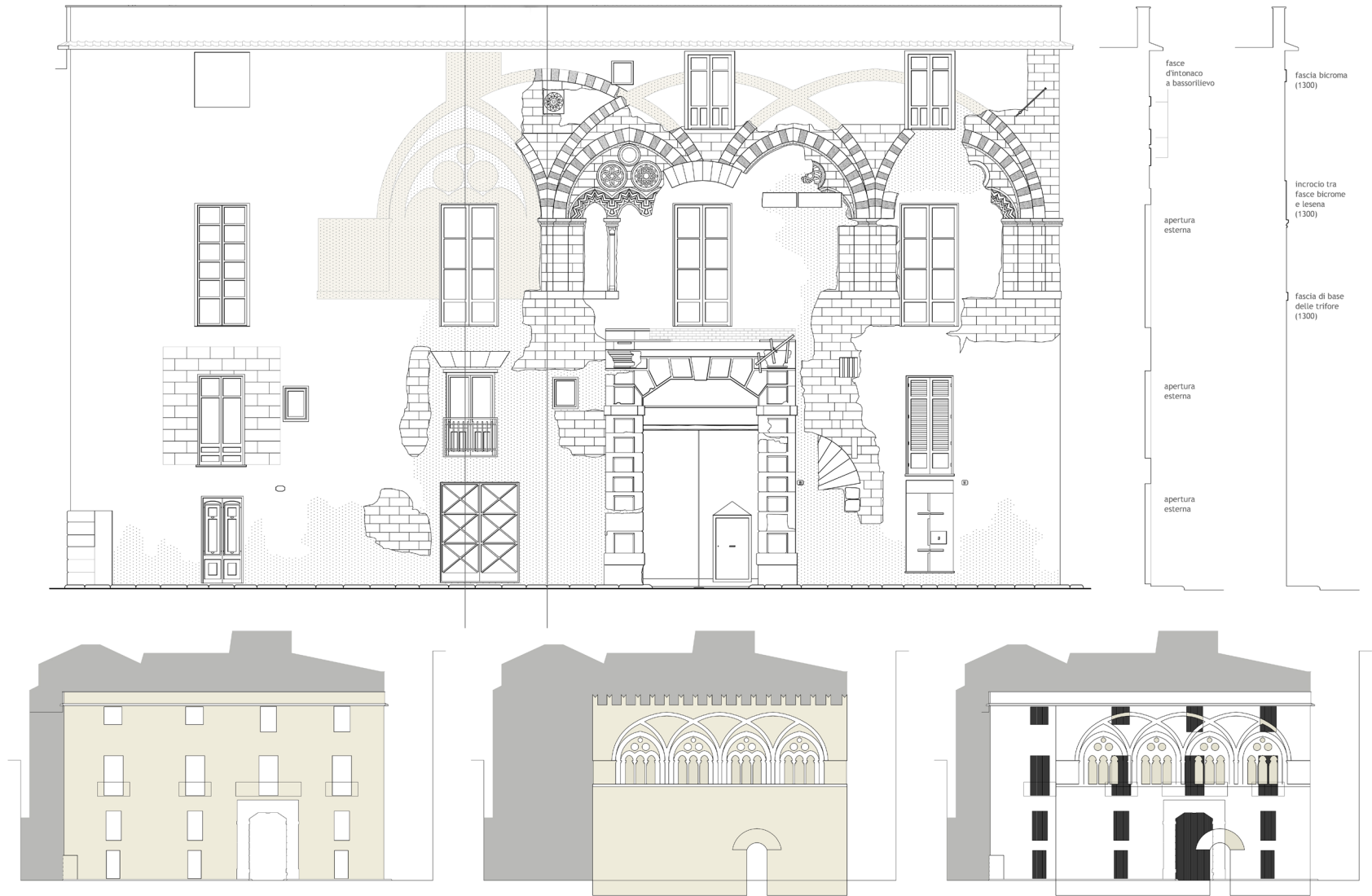
Fig. 12: Proposal for the restoration of Palazzo Cefalà in Palermo: preservation of all the architectural elements that can be attributed to each phase of the transformation of the building and critical reintegration of the gaps in the plaster. Below: graphic overlay between the nineteenth-century facade and the front view of the Chiaramonte tower-house (by the author).
